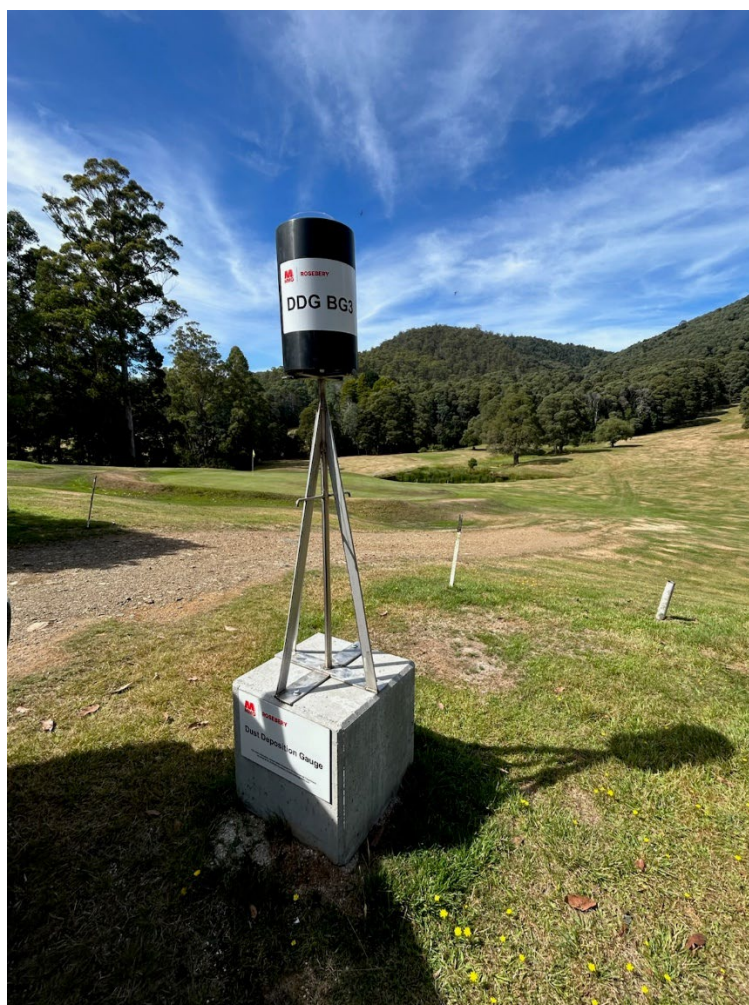
Figure 2. One of the upgraded dust deposition gauges installed across the Air Quality Monitoring Network.
