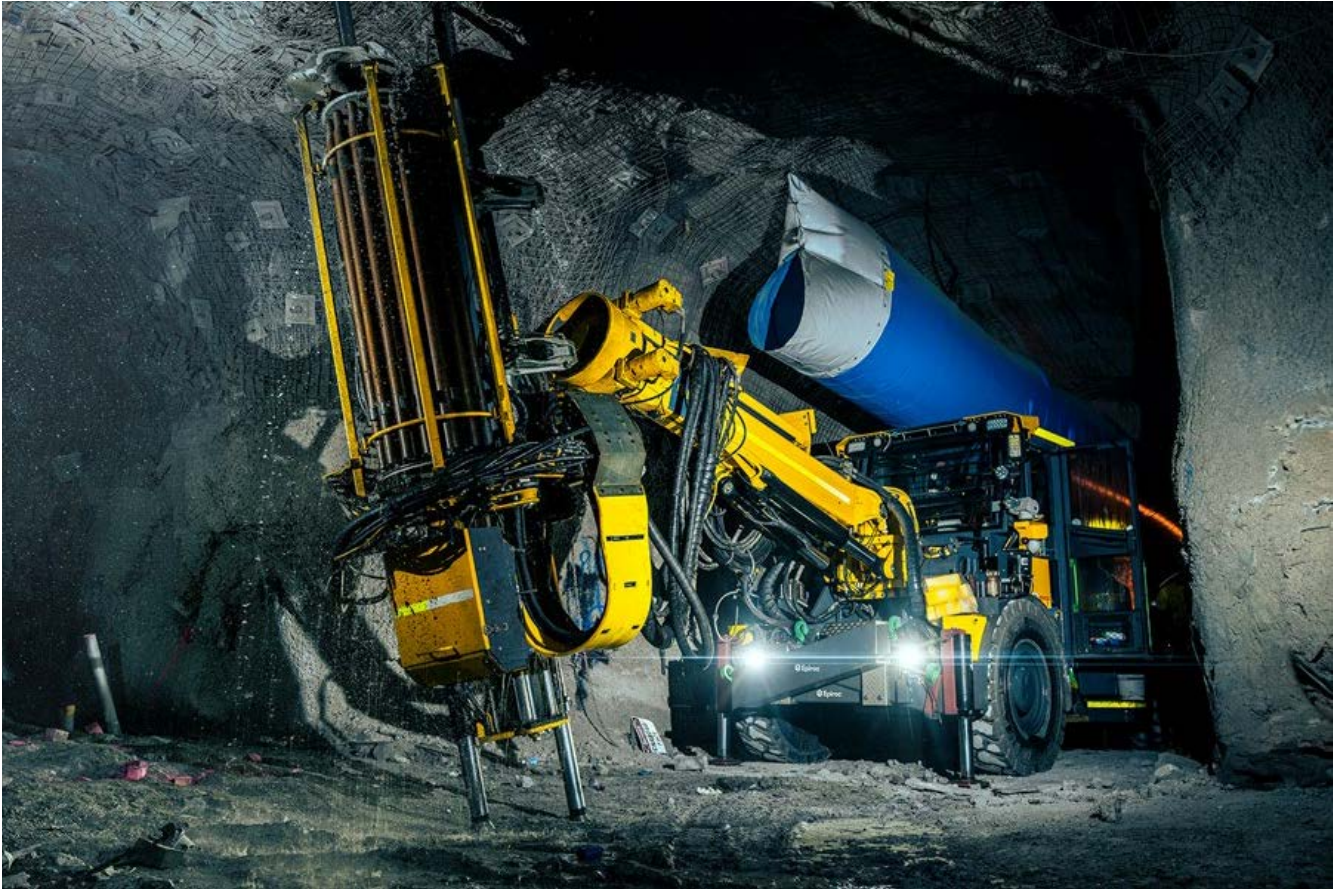
Figure 4. MMG Rosebery's Epiroc Simba E70SG replaced diesel with battery power.
