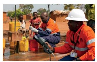
Water quality testing at a village bore pump as a part of baseline environmental monitoring.
