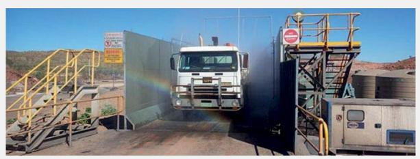
A truck washing station is used at Century to remove hazardous lead dust from vehicles.
