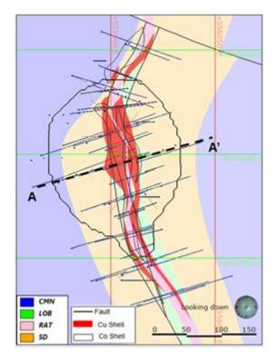
Figure 6: DZ geology and copper & cobalt grade shells. The dashed line designated A – A' is the location of the cross section shown in the following figure.
