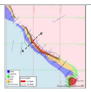
Figure 3: Nambulwa Main geology and copper & cobalt grade shells. The dashed line designated A – A' is the location of the cross section shown in the following figure.
