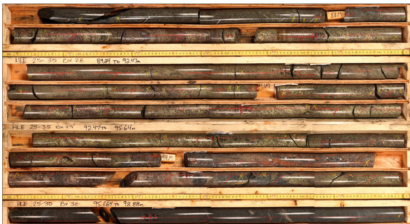
Figure 3. High Lake East drill hole HLE-25-35 intercept from 87m to 96m, 9m at 8.3% Cu, 9.5% Zn, 4.7 g/t Au and 123 g/t Ag.
