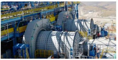
140ktpd throughput design capacity with two SAG and ball mill trains working independently of each other, pebble crusher and regrind circuit.
