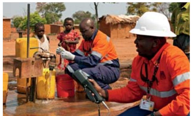
Water quality testing at a village bore pump as a part of baseline environmental monitoring.
